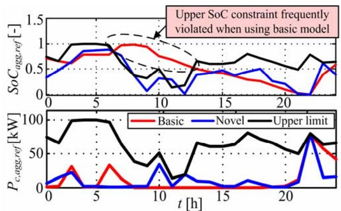
**DP-optimised aggregate battery charging power and SoC daily time profiles.**
