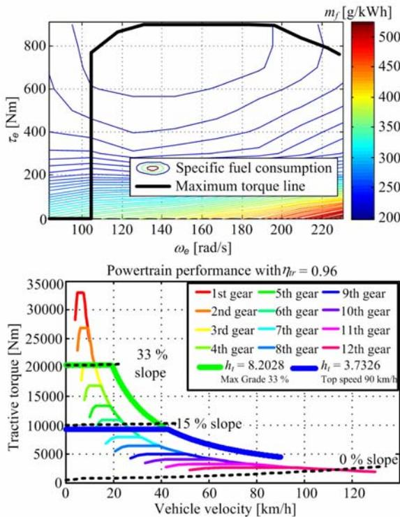
*Delivery truck diesel engine maps (upper subplot) and comparative torque limit curves for conventional and electric truck drivetrains (lower subplot).*
