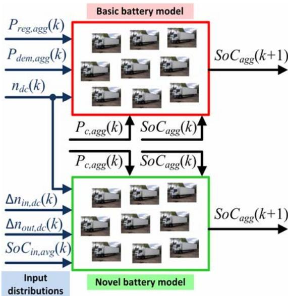
**Illustration of basic and novel aggregate battery models including corresponding input distributions, control and state variables.**
