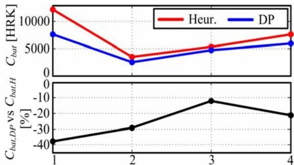
Comparative DP vs. heuristic algorithm results on aggregate battery charging costs for three months period and four electricity price models.
