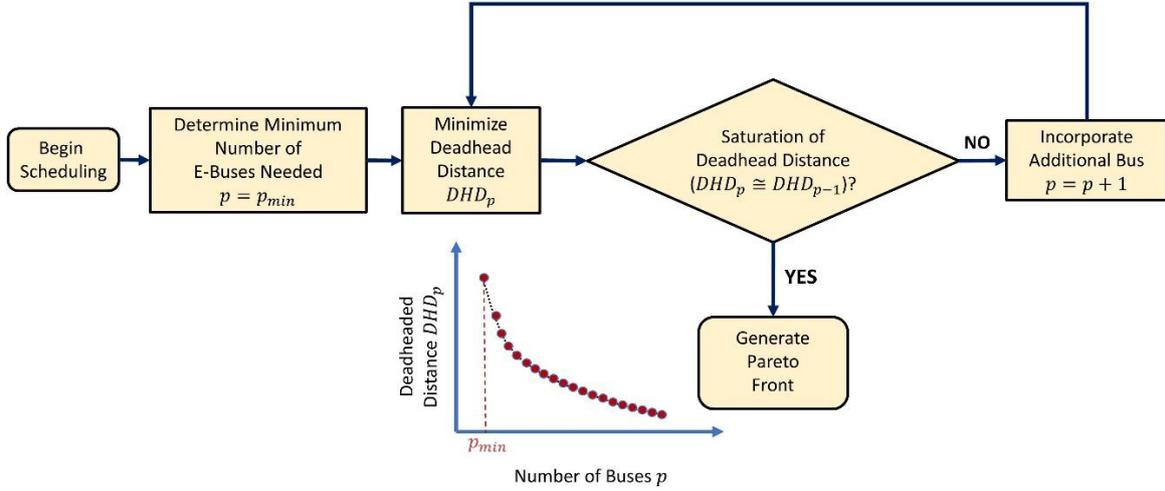
Fig. 1. Flowchart of e-bus scheduling sequential optimization process.
