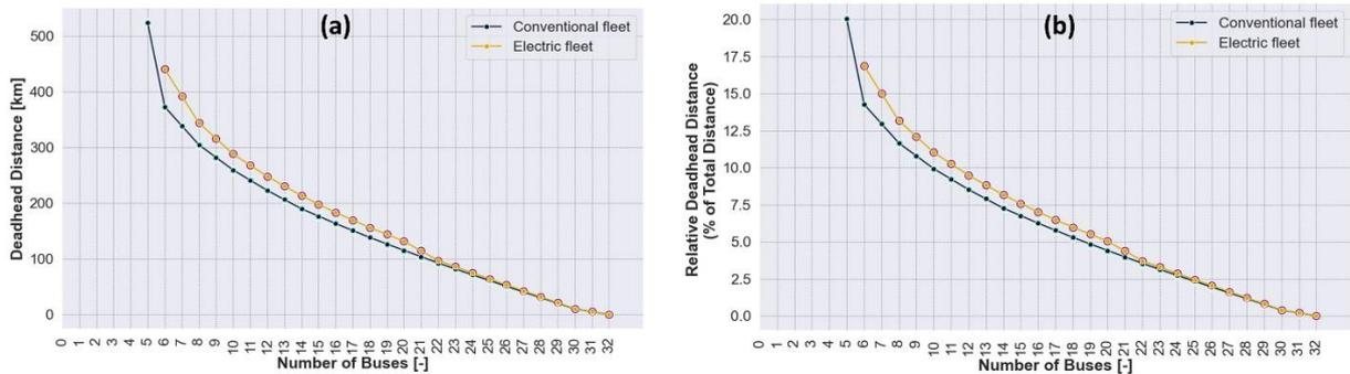
Fig. 3. Comparative Pareto frontiers obtained by MILP approach in the case of conventional and electric bus scheduling optimization.
